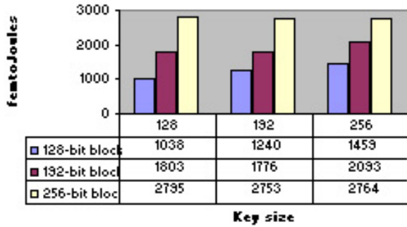
Fig. 7. Estimated energy used to encrypt 128 bits of data with AES
