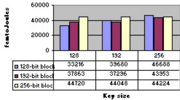
Fig. 10. Estimated energy used to encrypt 500 bytes of data with AES
