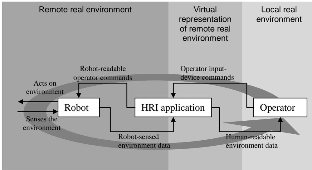
Figure 1: Simple representation of interaction cycle between robot and operator in an HRI system.
