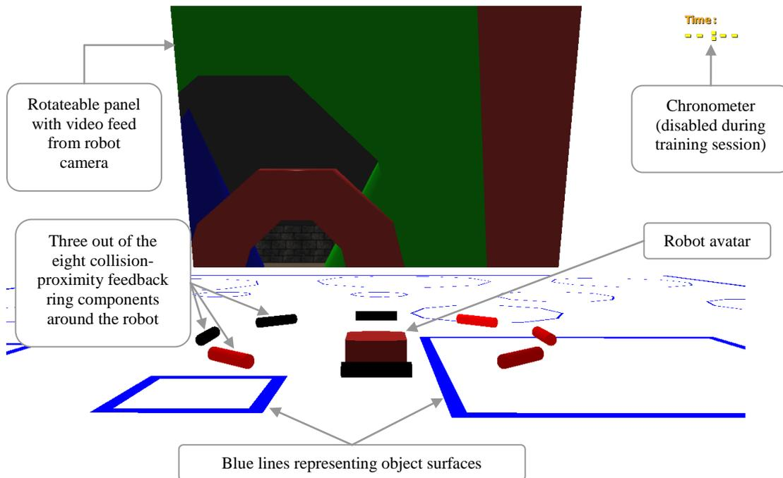
Figure 3: Main Components of the graphical interface.
